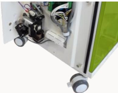
The integrated compressor kit provides the air necessary for both the brushless micromotor and the 3 functions syringe. **OPTIONAL**
