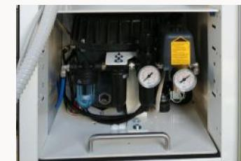
Oil compressor 24Lt. It provides air jet in support of pneumatic and electric rotatif instruments. **OPTIONAL**
