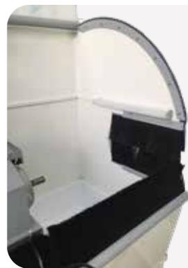
LED light sources assure a bright and total illumination of the working area without glare effect.
