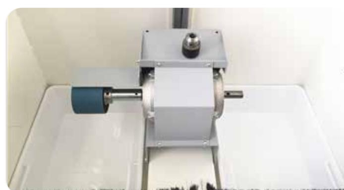
Dust and debris are collected in 2 plastic trays easily be removable.
