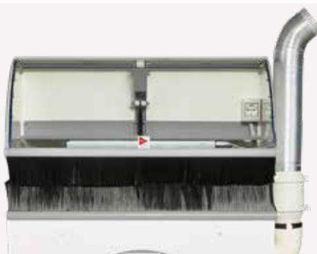
Provided with air extraction system and stainless steel pipe diam. 100 mm, length 350 mm.
