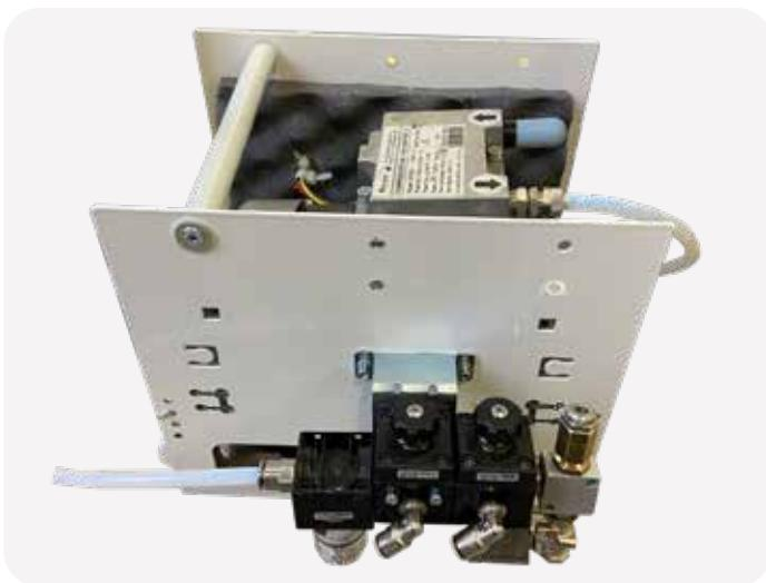
Integrated compressor inside the lower drawer of the storage, equipped with ventilation and soundproofing. It provides air jet in support of pneumatic and electric devices (70 l/min.).
