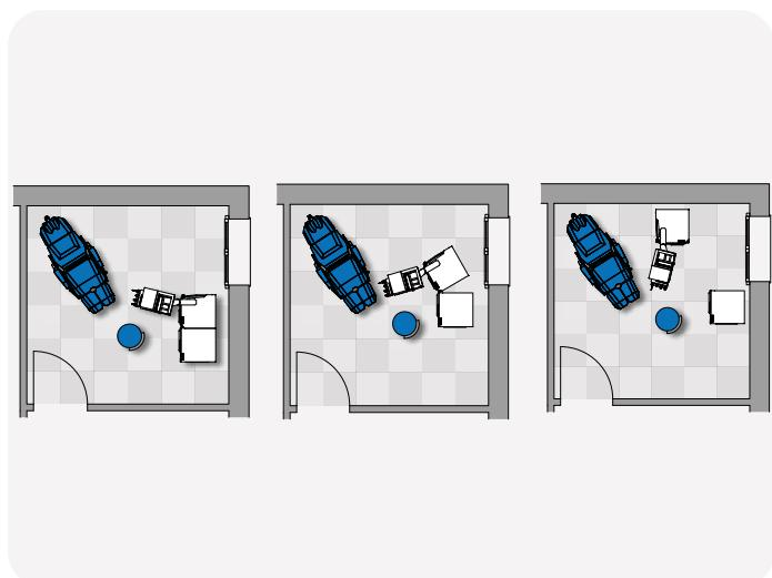
The two Cabinets are adjustable from 0 to 30 ° allowing the Operator to adapt the Unit to the available area. The rotation is guaranteed by steel bearings. The two sections remain attached by means of two electromagnets which can be released by the corresponding function activated by the touch screen.
