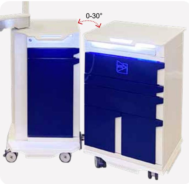
The two Cabinets are adjustable from 0 to 30 ° allowing the Operator to adapt the Unit to the available area. The rotation is guaranteed by steel bearings. The two sections remain attached by means of two electromagnets which can be released by the corresponding function activated by the touch screen.
