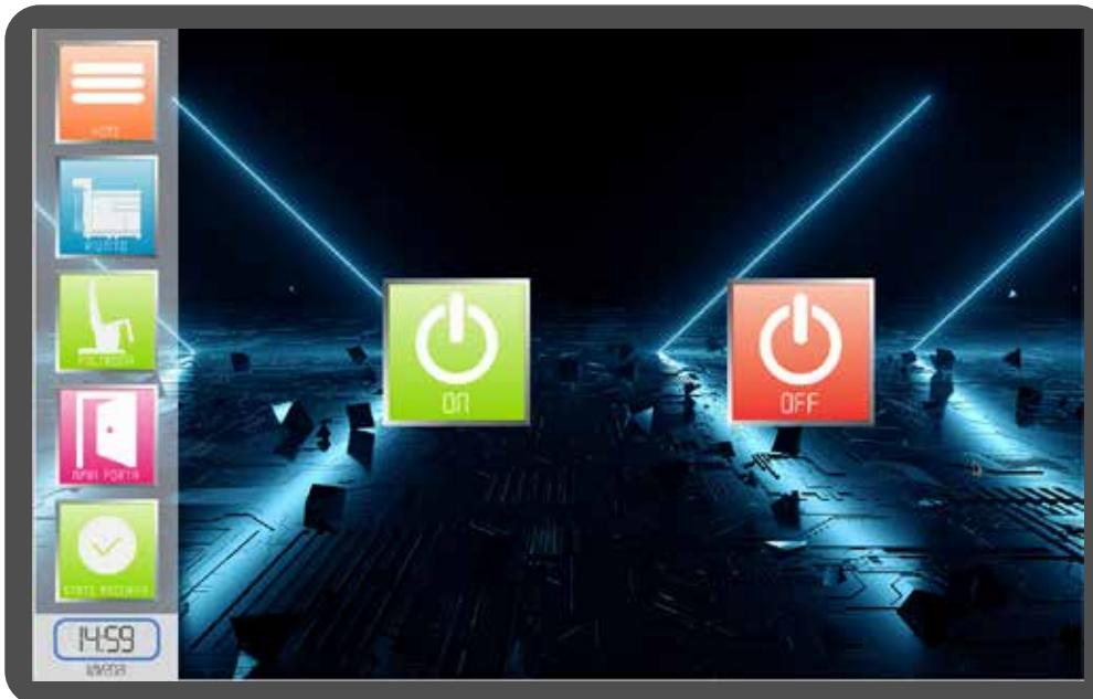
Thanks to the XBee radio frequency module, **INGENii** is able to control the Chair connected to the Unit, via the touch screen. From the panel it is possible to control single movements of the Chair, lock and recall the 7 memorized positions. During any single Chair movement, the touchscreen shows the operator the corresponding 3D graphics of that movement. It is possible to combine both the EDGE and MOTION range of Chairs.
