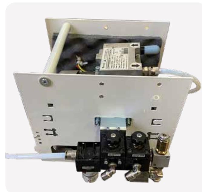
Integrated compressor inside the lower drawer of the storage, equipped with ventilation and soundproofing. It provides air jet in support of pneumatic and electric devices (40 l/min.).
