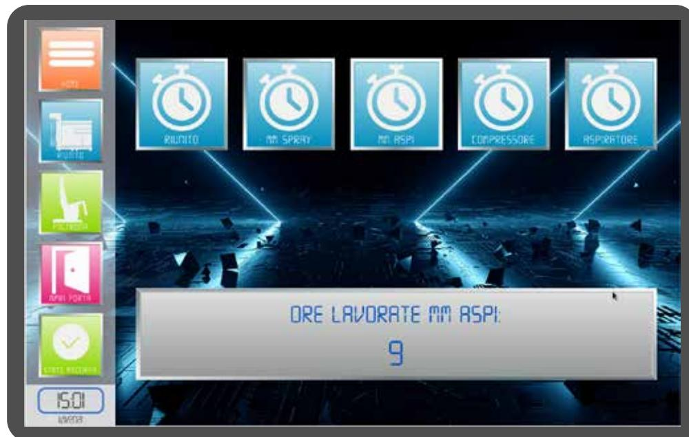
INGENii records hours worked by the Unit and main components into the Counter section. The number of hours is useful to schedule any maintenance activity.
